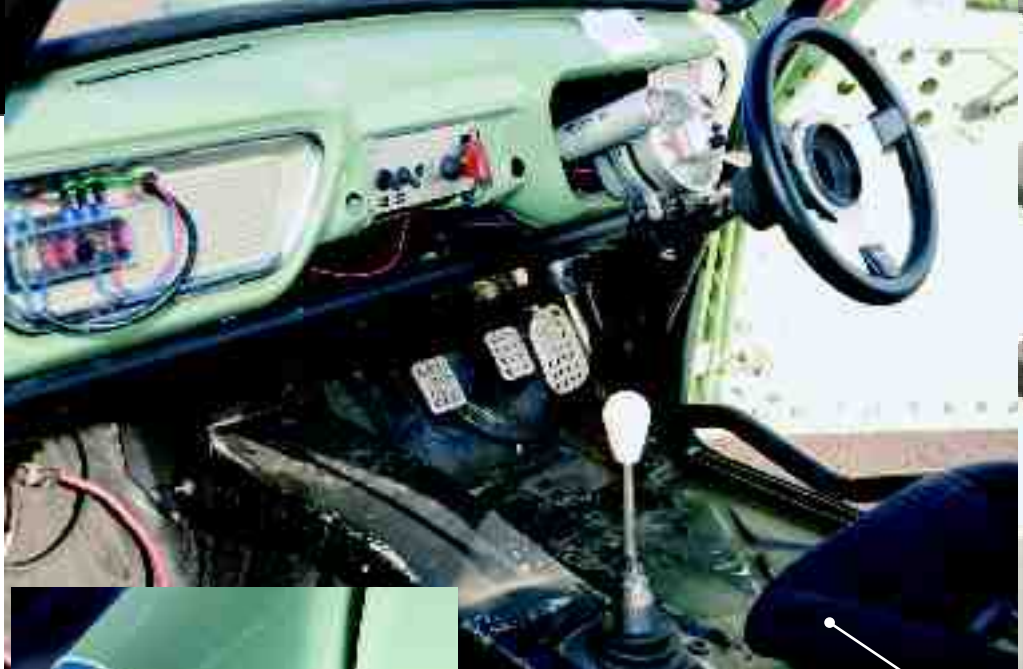
INTERIOR Totally stripped, Sparco 4 kg seat, Willans harnesses, alloy pedals, Mountney steering wheel, rev counter, roll cage — turreted for extra strength.
