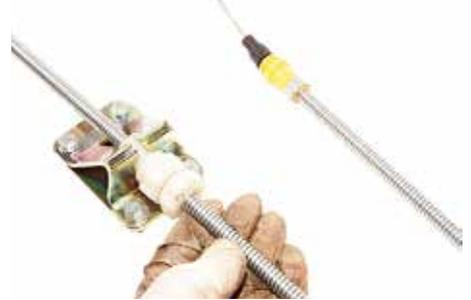
The adjuster sits in this bracket which is supplied with the kit and bolts into the transmission tunnel on the opposite side to the original tensioner bracket.
