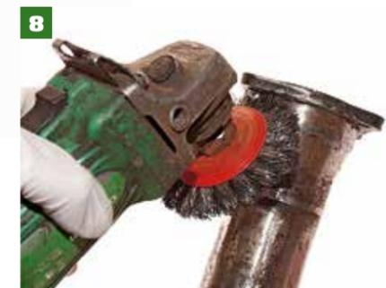
8 We need to fit our calliper mounting brackets next and there are three of them, so we cleaned up the seat area around the back of the end flange.
