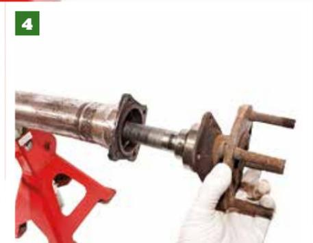
4 This allows us to pull the shafts free from the casing ready for machining.
