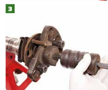
3 We still need to remove the halfshafts though, which we're doing with a slide hammer.
