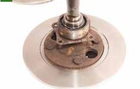
...as you can see, the halfshaft flanges are too big to go inside the Mk3 Fiesta solid discs that the kit uses.
