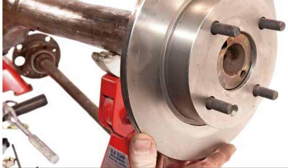
23 The discs go on next, which simply slide over the wheel studs — you can fit a wheel nut if you like to keep them in place for now.
