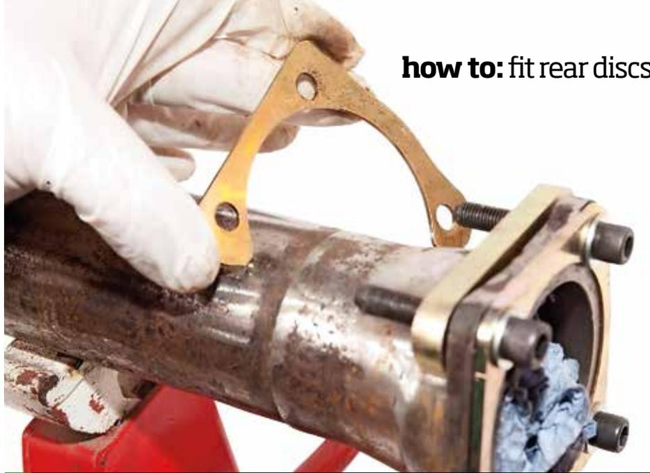
12 This thin spacer plate follows the first bracket, which in turn...
