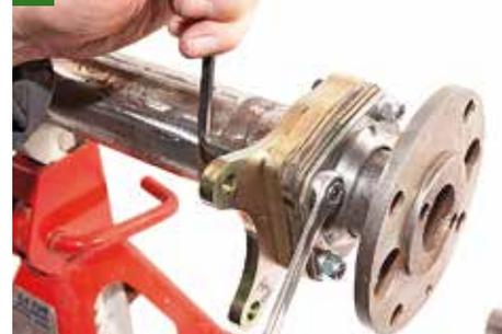
Then we fitted the halfshaft keeper plates over the protruding bolts, fitted the nuts and nipped it all up with a spanner and Allen key.
