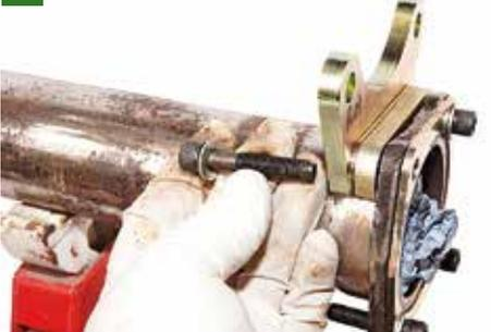
Before we can refit the shafts, we need to turn those bolts round; which we did one at a time so the lot didn't fall on the floor.
