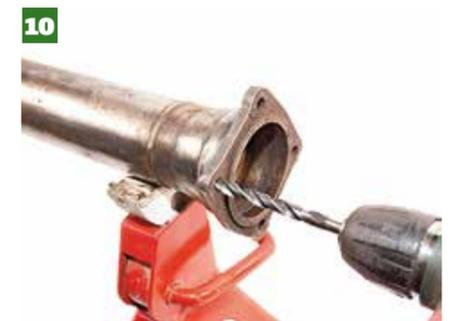
10 Anglia axles have threaded fixing holes in the mating flange, which need drilling out to 8 mm so that the new fixing bolts can be fitted.
