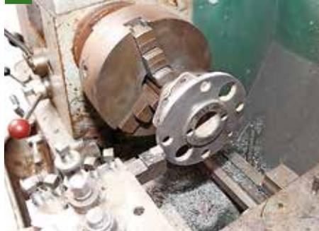
OFAS can provide halfshaft machining — we turned the flanges down to 132 mm.
