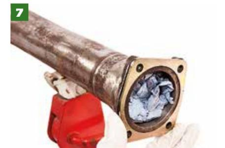
7 This spacer plate, which allows the halfshaft keeper plates to sit flush.
