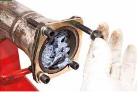
For now, we're fitting the supplied Allen bolts the wrong way round — it makes it easier to slide all the brackets on one by one.
