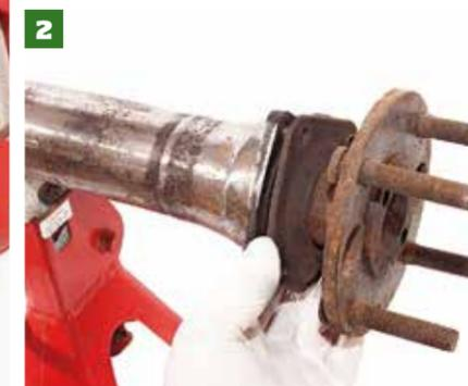
2 The flange plates are already loose as the brake backplates are missing — we'd normally need to unbolt these and remove the old brakes.
