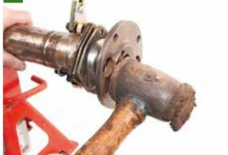
Next we slid the halfshafts into the casing and knocked them home with a copper/Hyde mallet, spread evenly across the flange face.
