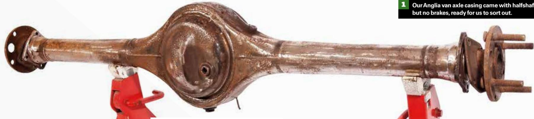
1 Our Anglia van axle casing came with halfshafts but no brakes, ready for us to sort out.
