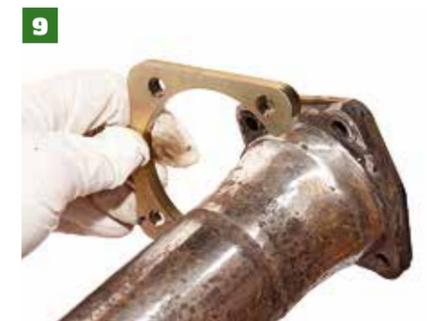
9 Ours needed some dressing to allow the first of the plates — this spacer — to fit flush.
