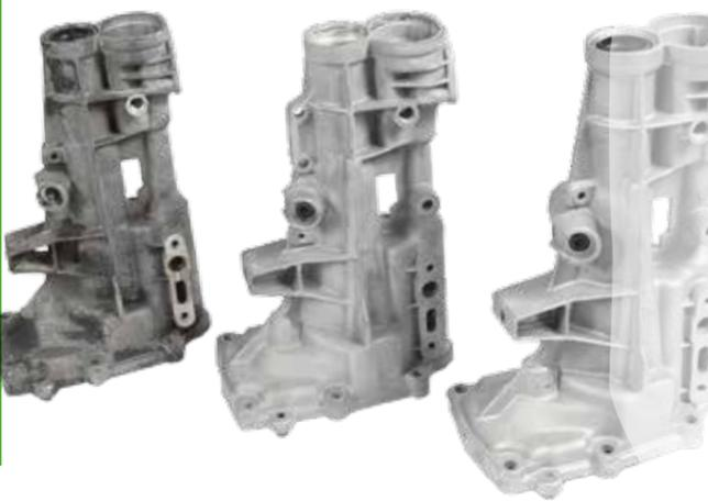
Over the course of the Type-9's production run, the design of the alloy tail casing was altered slightly. As has already been mentioned, later ones (middle and left) feature a extra rib that hides an oilway on the left-hand-side looking from the front. Some later ones also feature an additional bracket on the lower back (middle casing) to hang a weight on to help reduce noise and vibration. This is not required when you come to fit a Type-9 to your classic Ford.
