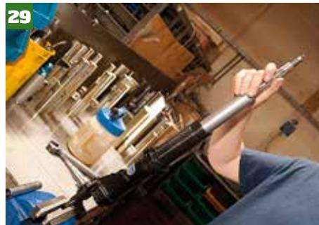
29 The unit can now be put into the strut body casing....
