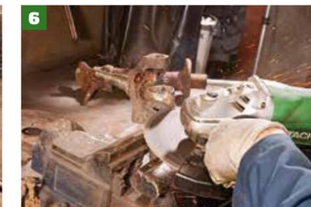
**6** Next, Mark mounts the strut upside down in the vice, and cuts the bottom of the strut body tube off with a disc cutter in an angle grinder, corresponding with the angle of the stub axle casting...
