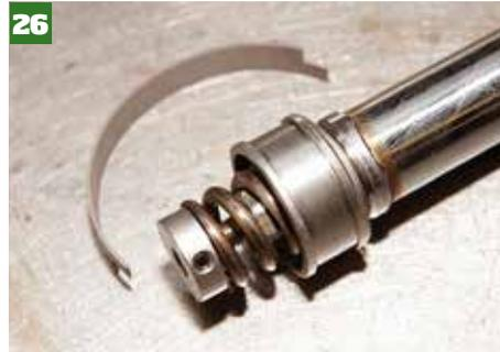
26 At the base of the rod is the piston assembly — to the side is the piston ring/seal...
