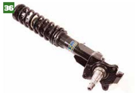
36 The struts are complete although we need to fit adjustable top mounts, which we'll discuss when we fit the struts to the car. We will also show how to adjust the struts for height and damping.
