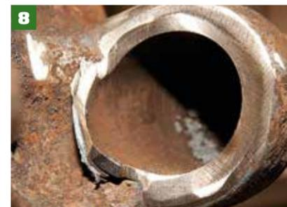
**8** If you look very carefully, you can see the very faint line that separates the casting with the strut tube, meaning it's no longer attached by weld.
