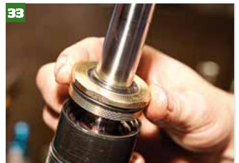
33 The fixing nut's added next and done up tight to seal the tube — damping system complete.
