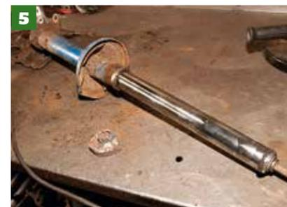
**5** Our Bilstein's a dry strut, meaning it has a self-contained insert that slots in the damper tube. It removes in the same way — undo the top nut and pull the insert out.
