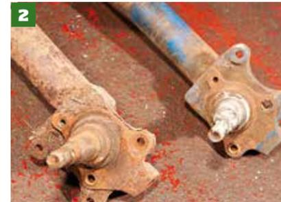
**2** We actually have an odd pair of struts — one's a 2-litre, the other a knackered Bilstein — but it doesn't matter for the aforementioned reason! Check the bearing surfaces are not pitted.
