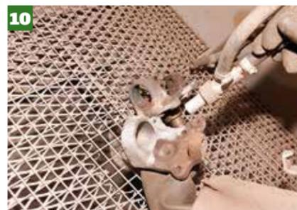
**10** The next step in Gaz's process — obviously, once they've cooled! — is to clean the stub axle castings up by shot blasting them. Don't touch the bearing surfaces, though!
