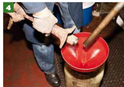
**4** Our 2-litre Capri strut is a wet strut, meaning the piston and rod is assembled in the casing along with the damping oil, which needs draining out into a suitable waste container.
