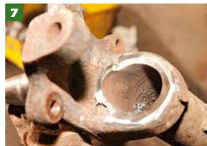
**7** ...he then dresses the weld back with a flap disc in a smaller grinder, again to the shape, so that you should end up with the tube flush with the stub axle casting...
