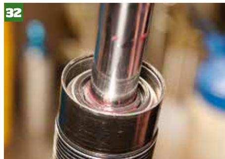
32 This sits just below the fixing nut along with a wiper seal, which is now fitted in place along with a twin-sprung, self-aligning, dual-lipped seal.
