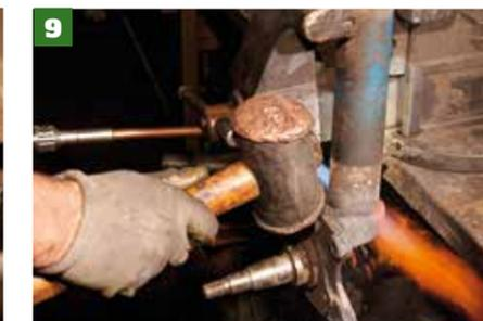
**9** Mark now heats the casting with an Oxy-Acetylene torch until it's red. A quick whack with a copper-faced hammer and the casting should drop to the floor — obviously, this needs care.
