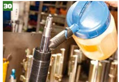
30 ...and high-viscosity, multi-grade damping oil is added to Gaz's own spec.
