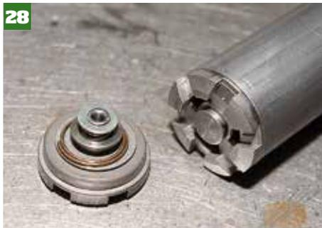
28 At the base of the tube is the valve assembly, which simply pushes into the base of the pressure tube.
