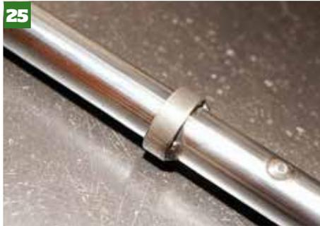
25 ...onto which, the stops correspond. This is pretty simple — Gaz machine a steel ring, which is slid over the rod and is welded in place with two sections of stitch-welded MiG.
