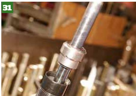
31 The top's sealed with the rod guide which supports the piston rod is first fitted at the top.
