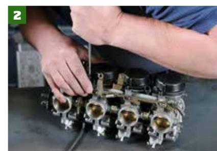
2 Begin by unscrewing the carb tops — make sure you use a good fitting screwdriver to avoid damaging the threads as these are often tight. Carefully lift out the spring, diaphragm and sliding needle assembly.
