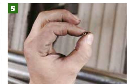
5 Remove the smaller pilot jets with a good fitting flat bladed screwdriver. These only need to be checked for dirt or blockages so hold them up to light and check. Clean through carefully with the strand of a wire brush if it needs it.
