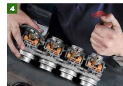
4 Remove the main jets, again using a good fitting flat-bladed screwdriver. These are the jets that need to be enlarged. Steve suggests drilling them out to 1.6-1.7 mm as a starting base so carefully use a drill and a vice or borrow a pillar drill.
