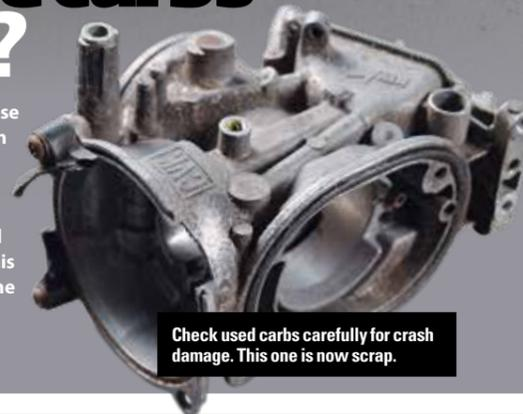
Check used carbs carefully for crash damage. This one is now scrap.
