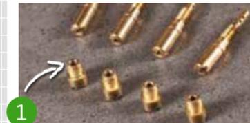
1 Once the carbs have been stripped and cleaned they need to be drilled out to the correct 1.6-1.7 mm, which Steve recommends as a good starting base. They then need to be reassembled carefully and if you are not using a bike fuel pump then make
