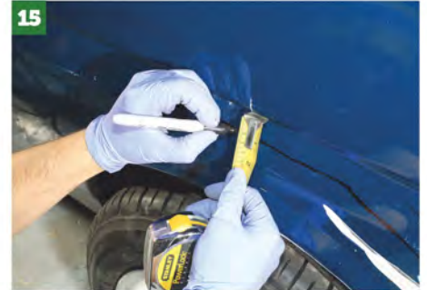
15 The next bit's the point of no-return! Matt has marked a line around the outside of the arch, then removes it and marks another inside it, but 20 mm further down.
