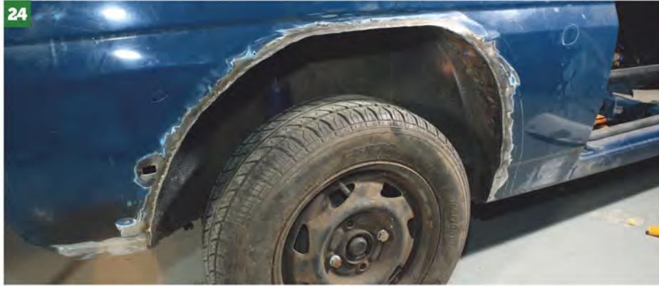
Matt's worked his way round until the arch is completely shut...
