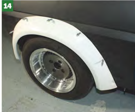
14 It goes without say that Matt also fitted the rally arch to the front as well, using Clecos.
