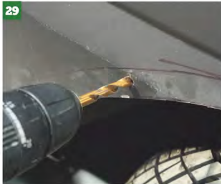
All you need to do is drill a clearance hole into the arch, using the Cleco fixing hole as reference.
