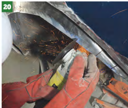
20 Next we need to reshape the inner arch to meet the outer, so Matt cuts thin slots into the inner skin...
