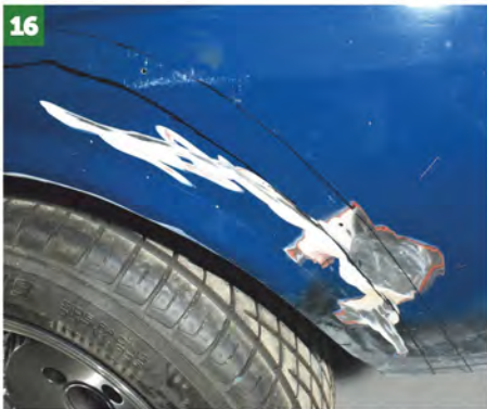
16 He works his way around the whole arch until all the marks are joined up — this is his cut line!
