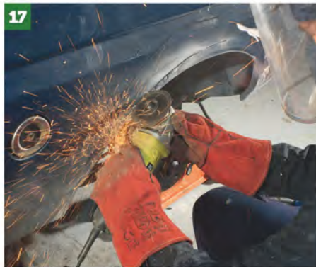
17 Using a 1 mm cutting disc in an angle grinder, Matt carefully cuts through the outer skin...
