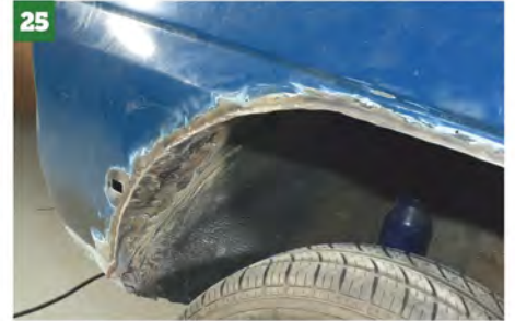
...and then dressed the welds back so they're nice and neat — he'll apply some seam sealer later plus some stone chip to protect the steel from corrosion in the inner arch when the time comes to finish the car.
