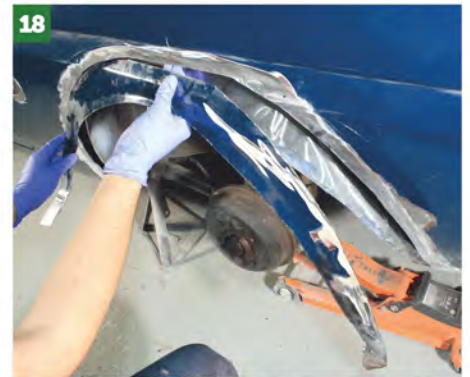
18 ...and trims off the bottom of the arch so that the outer skin comes away...
