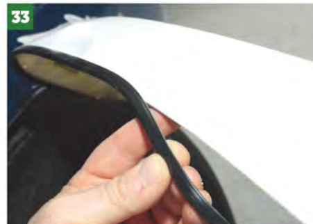
He's left it off for now but Matt has also sourced a plastic U-section strip to finish the edges of the arch — this simply slides into place and serves to hide the gap between arch and wing.
